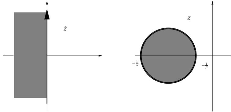
For  $\tilde{G}(s)$  to be (strictly) positive-real, we also need it to be asymptotically stable. But  $\tilde{G}(s) = 1 + \frac{(\beta-\alpha)G(s)}{1+\alpha G(s)}$  and this transfer function is stable if the feedback combination of  $G(s)$  and  $-\alpha$  is stable. By the Nyquist criterion, this will be the case if the locus of  $G(j\omega)$  encircles the point  $-1/\alpha$  as many times anticlockwise as  $G(s)$  has unstable poles. Putting all this together gives:
