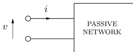
Passivity of the network means that it can only absorb power. Formally: a network is passive if for all square integrable pairs  $v(t)$  and  $i(t)$  and all  $T$  then  $\int_{-\infty}^T v(t)i(t)dt \geq 0$ . This readily gives a necessary condition on the impedance as follows.
