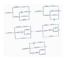
5 networks with 3 reactive elements and (at most) 5 resistors
