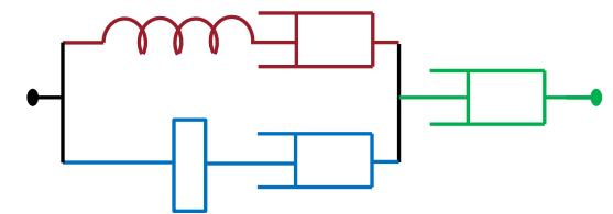
Stage C: Remaining resistors/dampers are connected in series or in parallel
