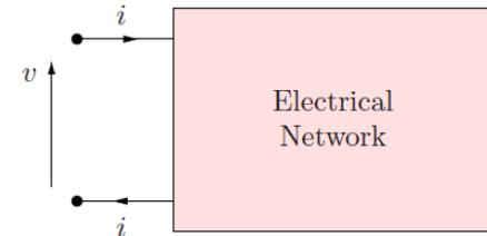
O. Brune showed that any positive-real function could be realised as the impedance or admittance of a network comprising resistors, capacitors, inductors and *transformers*. (1931)
