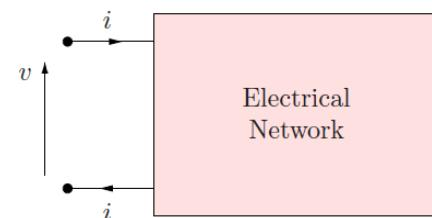
O. Brune showed that any positive-real function could be realised as the impedance or admittance of a network Comprising resistors, capacitors, inductors and *transformers*. (1931)
