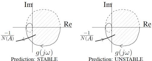
Stability: greater A should correspond to a point that satisfies the encirclement condition of Nyquist criterion, that is, oscillations of larger amplitude will be attenuated.
