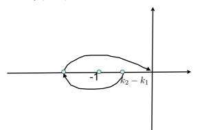
The describing function predicts a stable limit cycle for any nonlinearity such that N(0)=1 and with a monotone decreasing gain.
