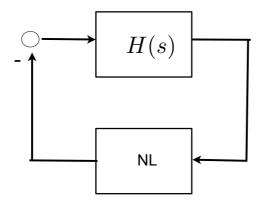
Approximating the static nonlinearity by an equivalent frequency-dependent gain (or transfer function)
