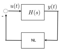
A limit cycle means that the feedback system admits a periodic behavior (u(t),y(t)).
