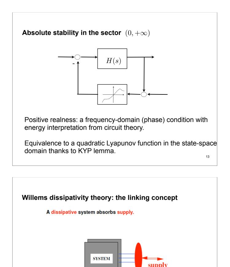
Lyapunov functions quantify the internal dissipation.
