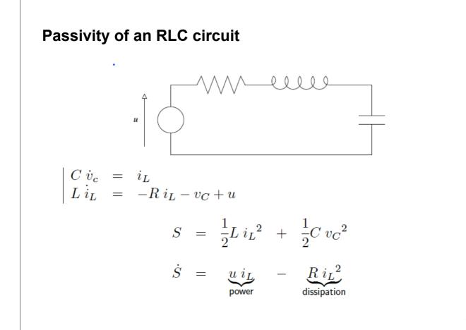
Link with the circuit concept of passivity
