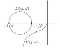
Compare with the necessary condition: the disk replaced by a segment.
