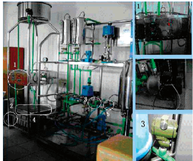
Figure 3. Constant pressure water supply system.
